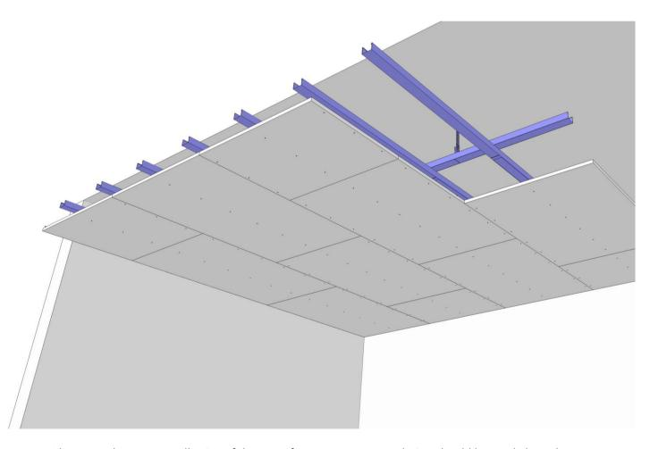
Where panels meet, an adhesive of the manufacturers recommendation should be used along the entire profile of the edge. Any adhesive that seeps out can be sanded level once dry. The same adhesive is used in the mechanical fixing holes and again sanded level.
