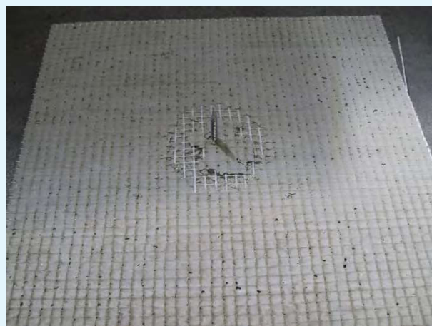
Example of failure with pull-out of screw
